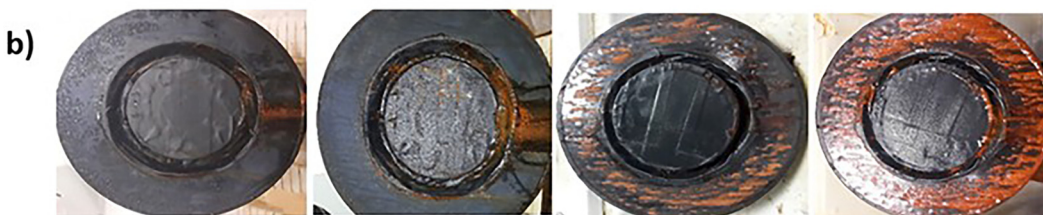
Figure 6: a) Comparison of corrosion resistance of uncoated and coated discs during the salt fog test, b) brake disc appearances with red rust observed during salt fog corrosion test.
